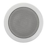
The Apart EN-CM6T6 is a 6" built-in ceiling speaker made of powder coated steel (RAL 9010 equivalent), equipped with a high efficiency full range speaker and a multi tap 100 volt transformer, all certified according EN 54-24. The unit is equipped with a ceramic speaker line connector block, thermal fuse and a metal fire dome.
